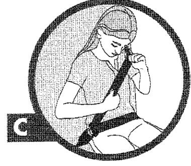
**C** TIGHTEN the lap portion by pulling upward on the shoulder belt. Be sure that the shoulder belt is snug across the chest and crosses the center of the shoulder.
